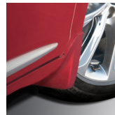
Molded Splash Guards / Rear Molded Splash Guards in Limited Addiction Red (G1E)
